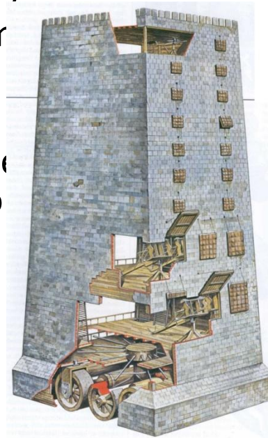
The Helepolis at Rhodes Height: 130-140R (40-43m) Base: 72R (22m) square Armament: Lower floor: 2x180 iber (82kg) catapults; 1x60 iber (27kg) catapult 1st floor: 2x60 iber (27kg) catapults Next five floors: 2x60 iber (4kg) catapults Top two floors: 2x dart-throwers. Construction: main beams are fir or pine, wheels and horizontals are oak. All major joints are reinforced with iron plates to protect the machine from fire missiles. Its exterior is clad with iron-plates on 3 sides. Propulsion: the machine is mounted on eight wheels each 14ft (4.3m) in diameter. It is propelled by a capstan and sail drive, with a suitable mechanical advantage. (manned by roughly 200 men). Additional thrust could be provided from the rear. Weight: Probably around 150 tons. Siege towers had existed since Assyrian times. That illustrated is the famous Helepolis built by Epimachus of Athens for Demetrius Poliorcetes (the Besieger) in 304 BC. This was the largest siege tower of ancient times and descriptions of it survive in the accounts of Vitruvius, Diodorus, Plutarch and the so-called Athenaeus Mechanicus. Most siege towers were smaller than this gigantic structure and were made of wood or hide and saw-wood covered. Many had drawbridges, but this one apparently did not. In action it was brought up within missile range of the walls, supplying suppressing fire against the defenders. The large stone-thrower could even destroy ramparts and curtain walls. Since this had been accomplished, attackers could bring up battering rams and drills, or undermine the walls. Alternatively an assault could be mounted with ladders, drawbridges, sambucos etc.
